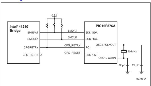
Figure 2. 41210 Bridge Microcontroller Connections
